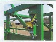
STEP 10 Remove winch which operates back butt strap.
