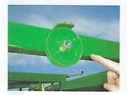
STEP 3 Pulley goes on front bolt.
