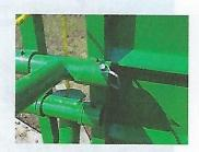
STEP 9 Lock arm in working position with clip pin.
